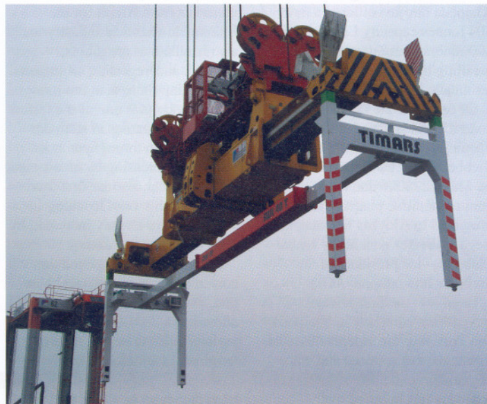
Interest in Timars’ latest invention – the automatic overheight frame (OHA) for handling flats or oversized containers is increasing all the time.
